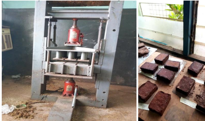
Fig. 1: Manual hydraulic press (9.5 MPa capacity) and briquettes
